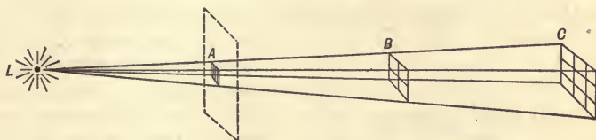
FIG. 201. — The Intensity of Light Varies Inversely as the Square of the Distance.
